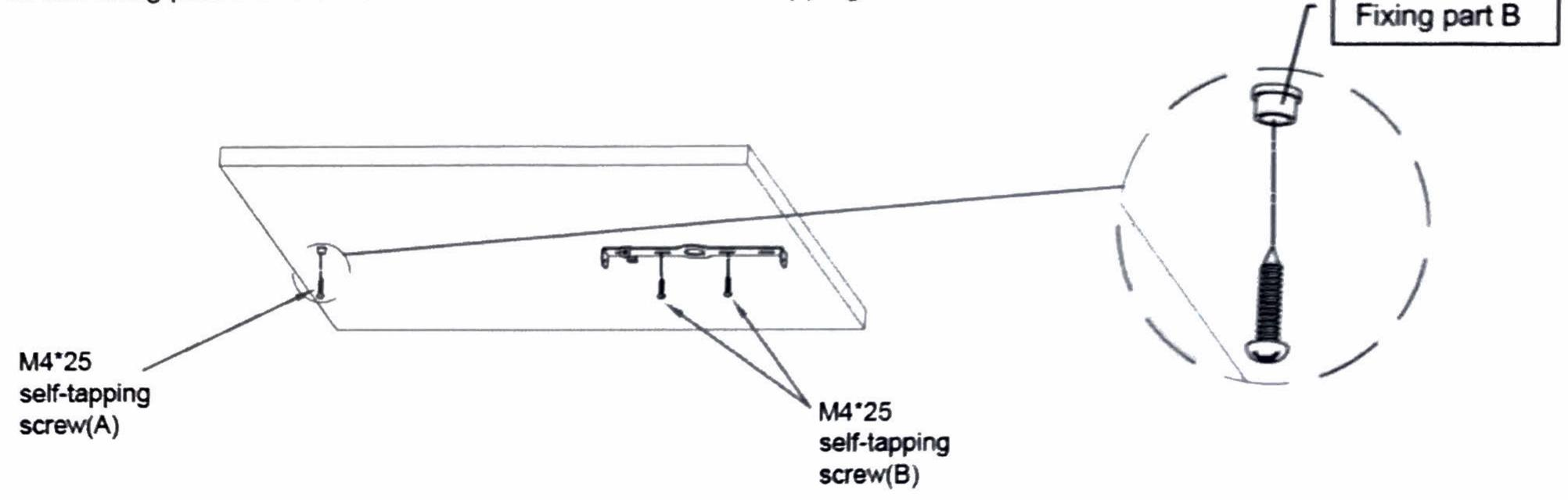
2. As shown in the following illustration, firstly, penetrate the steel rope B into regulator, and then turn fixing part A to fixing part B in the ceiling and 6 positions in the up side of the fixture.
