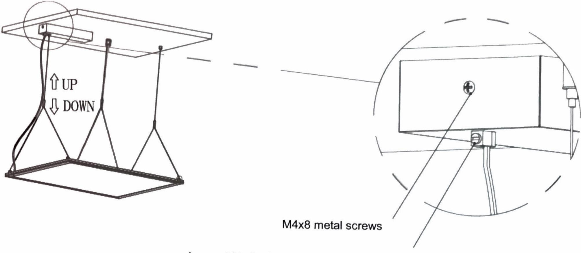
loosen M4 plastic screws to adjust the length of the wire
